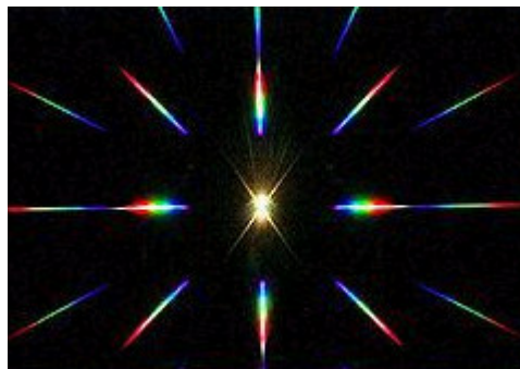
Figure 2. A white light source observed through a crossed transmission diffraction grating with a groove density of 530 lines/mm.
